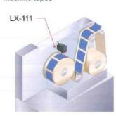
Detection of tapes stuck on copper foils
