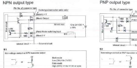
Layout of connector pin for connector type LX-111 □-Z
